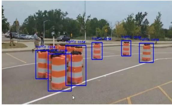
Figure 6. Traffic cone detection
