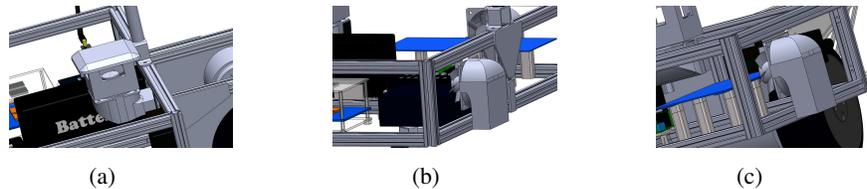
Figure 3: Three cooling fans.
