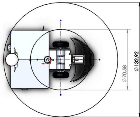
Figure 6: Novel maneuverability via minimizing the turning radius of the robot.
