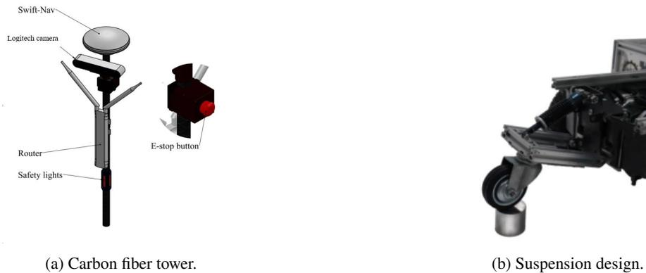
Figure 9: Carbon fiber tower and suspension design.
