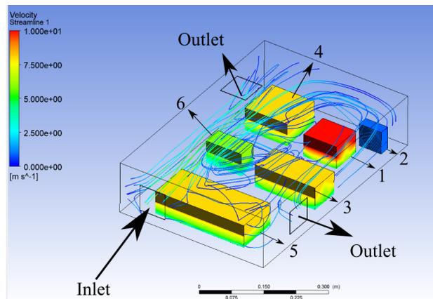
Figure 4: Heat distribution of cooling system. 1- Motor drivers, 2- Arduino, 3- Battery, 4- NUC, 5- PCB, 6- USB HUB.
