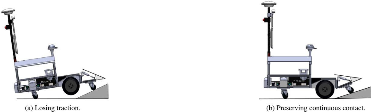
Figure 7: Motion of our robot when ascending uphill.
