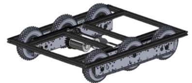
**Figure 5:** The chassis design allows turning at the center of mass and easy traversal of ramps.
