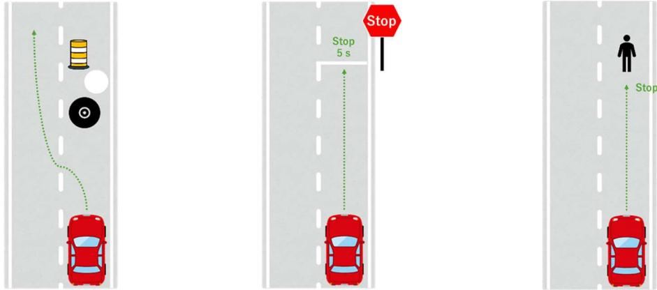
(a) When a tire or pothole is recognized, the vehicle deviates from the dashed line to avoid the obstacle.
