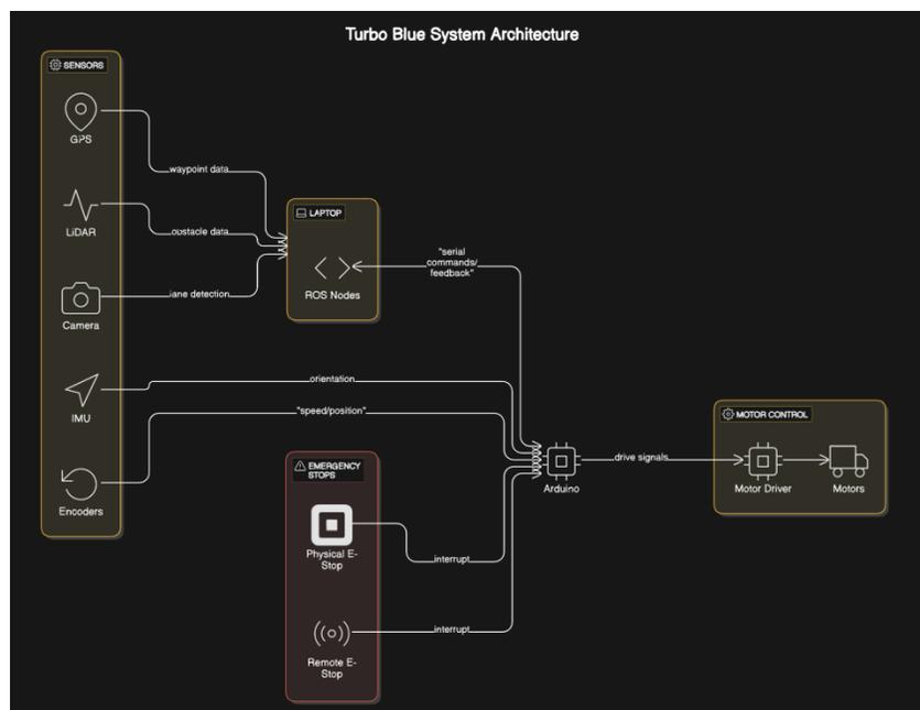
Figure 1. Turbo Blue System Architecture.
