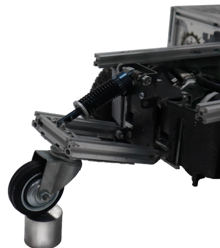
Figure 10: Spring action during uphill
