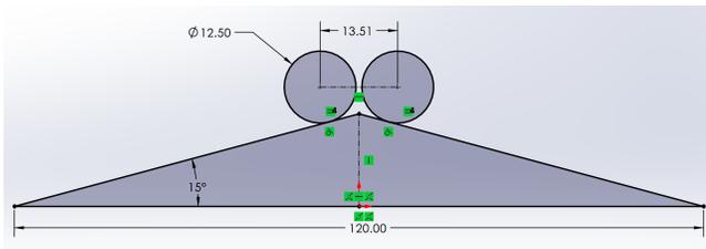
**Figure 11.** Simulation to determine wheel base for traversing the incline.
