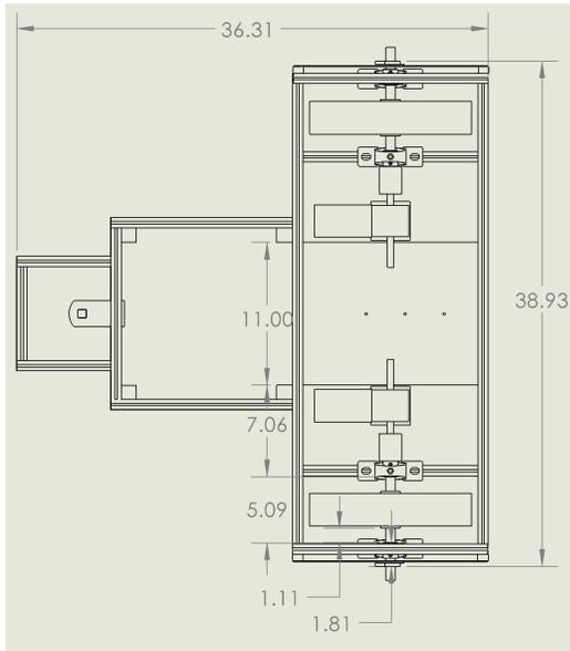
**Figure 10.** Length and width dimensions of the 2024 IGVC robot.
