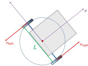
**Figure 13.** Turning radius provided by a differential robot design.
