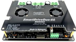
**Figure 8.** Motor controller utilized for the 2024 IGVC robot.
