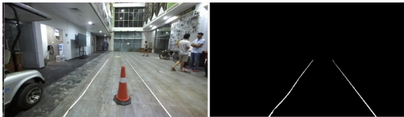
Figure 19: Lane Detection using OpenCV
