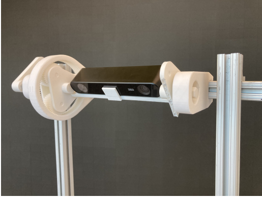
Figure 9: Mounted ZED camera
