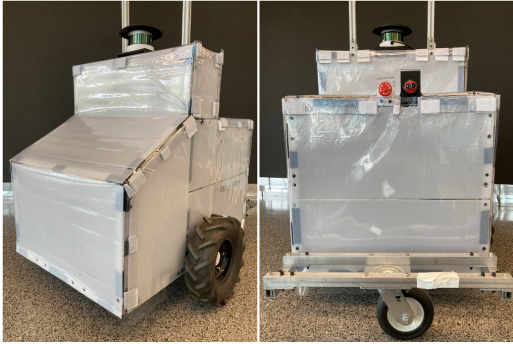
Figure 7: A demonstration of the raincoat protecting the electronics stack while not limiting function
