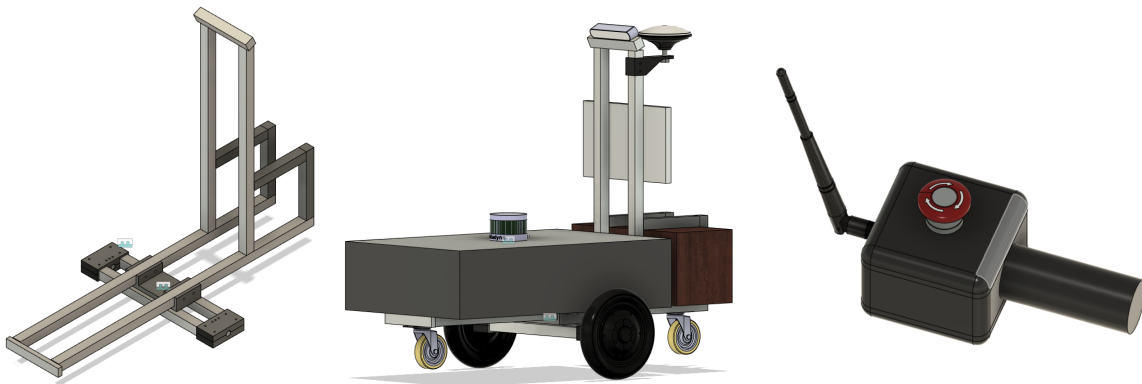
Fig 2, 3 & 4 : Bare Chassis, Complete Chassis, Wireless Electronic Kill Switch
