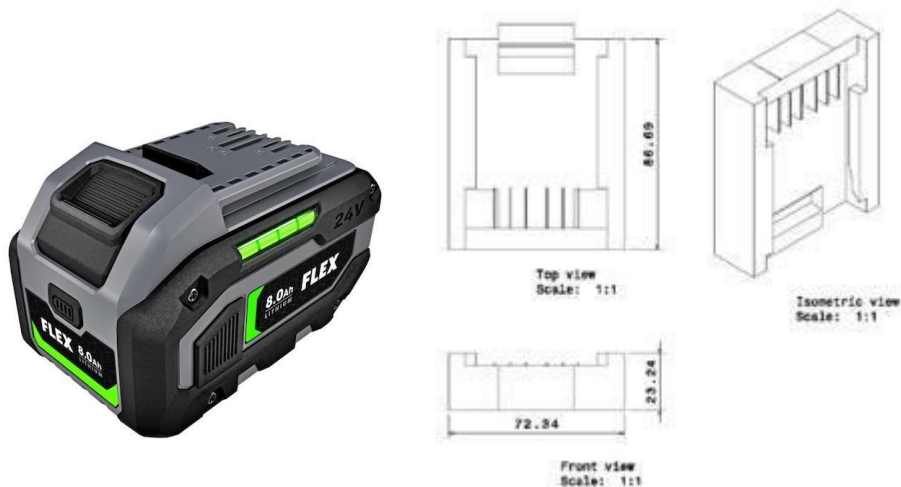
Figure 10: CAD Drawing of Battery Mount
