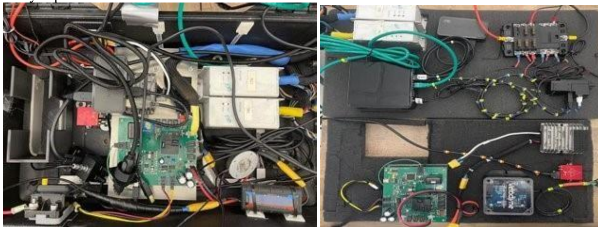
Figure 2 – Before and after wire organization
