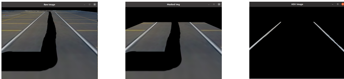
Figure 10. Left to Right: Raw Source Image, Masked Source Image, HSV Filtered Image
