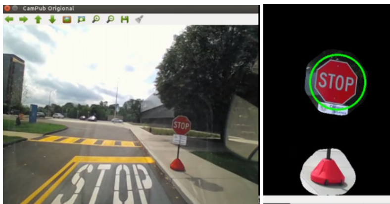
Figure 12: An example of detecting a stop sign
