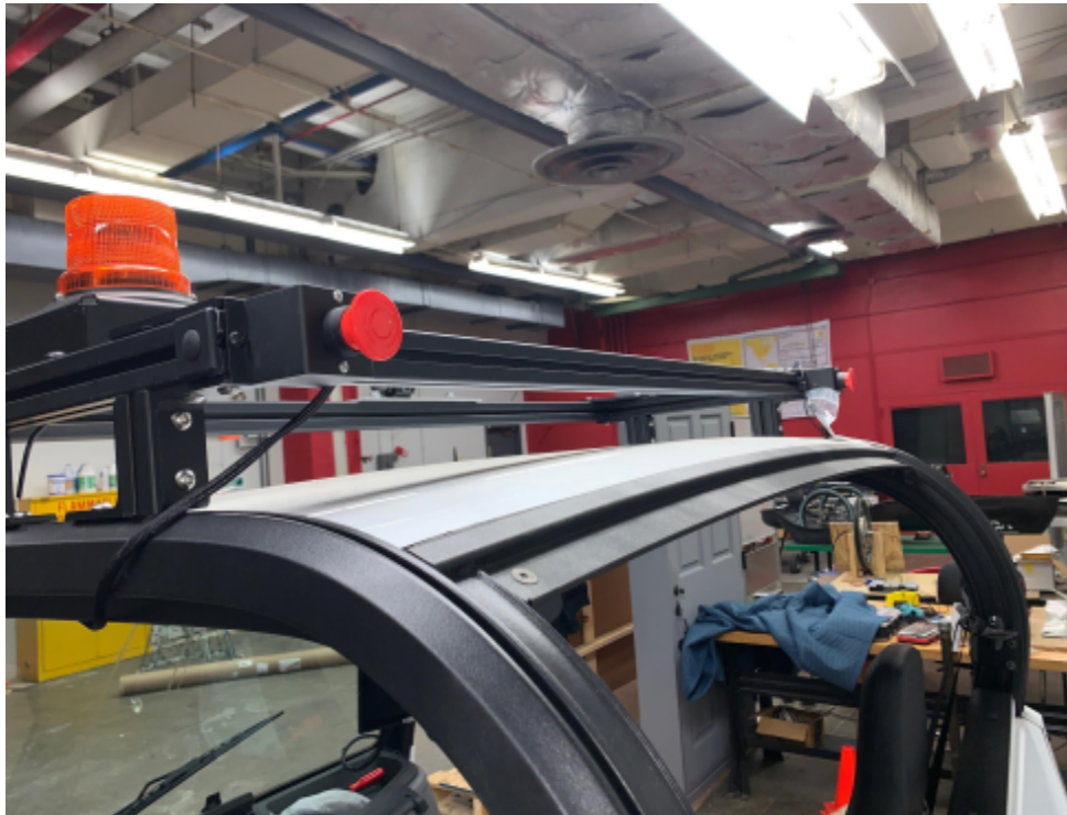
Figure 2.3: Safety light with Top Mounted Wired E-Stops, used to shut off the autonomous mode and give control to the fallback driver.
