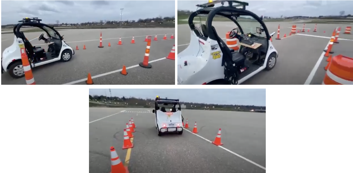
Figure 4.3: Pictures of the vehicle completing a turn-right functional navigation test.
