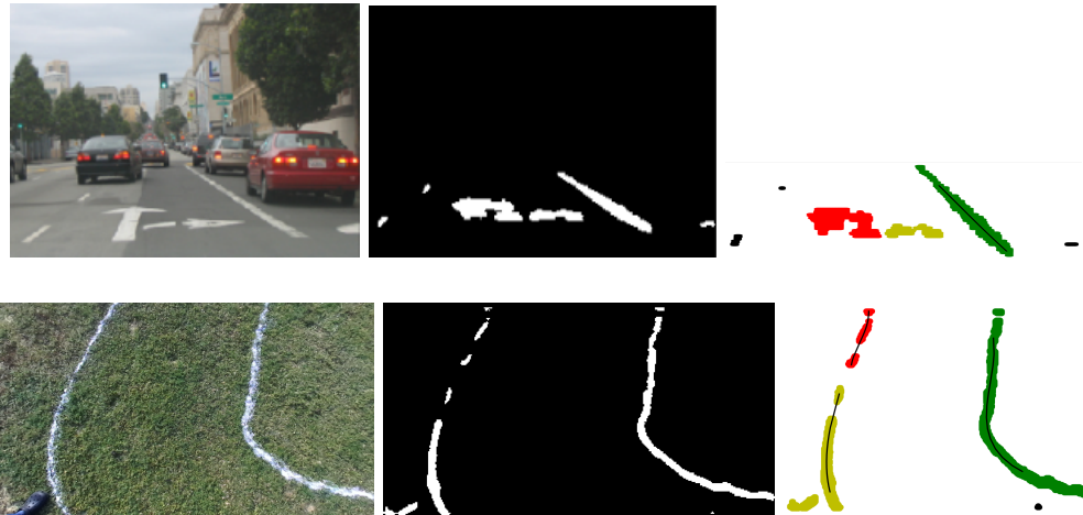
Input, corresponding output of UNET segmentation model, and fitting of output (the lanes with an appropriate fit are drawn in black)
