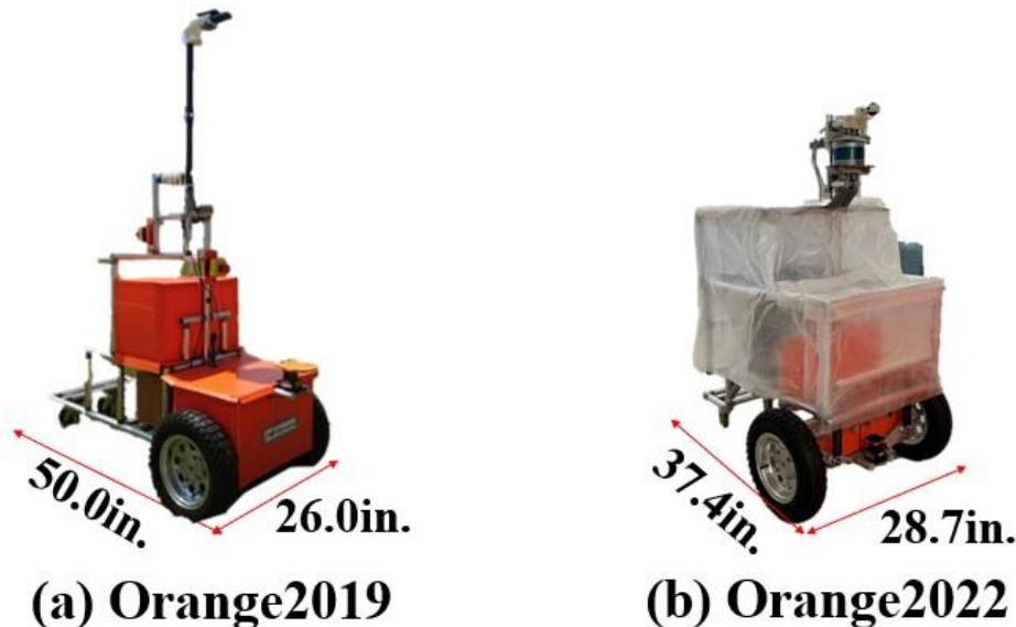
(a) Orange2019 (b) Orange2022 Figure 5. The design comparison between the Orange2019 and Orange2022 vehicle body
