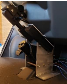
Figure 1: The Parking Brake Actuator with its Housing
