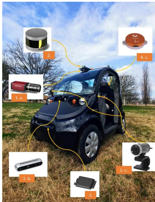
Figure 5. Sensor locations in the vehicle.
