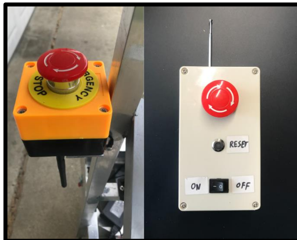
Figure 10: Mechanical E-stop (left) & Wireless E-stop (right)
