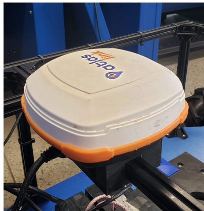
Figure 12: GPS receiver mount.
