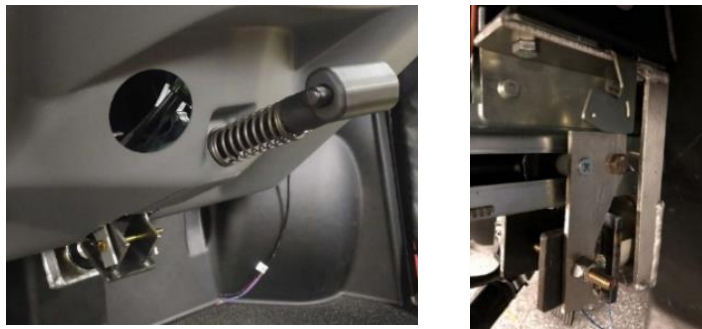
Figure 10: Stock-issued Braking Mechanism
