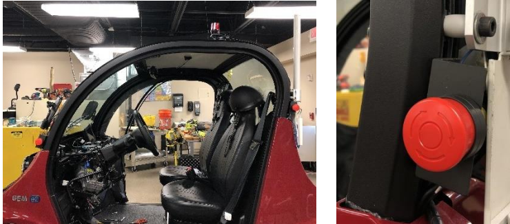
Figure 12: Emergency Stop Buttons Drive-By-Wire Conversion
