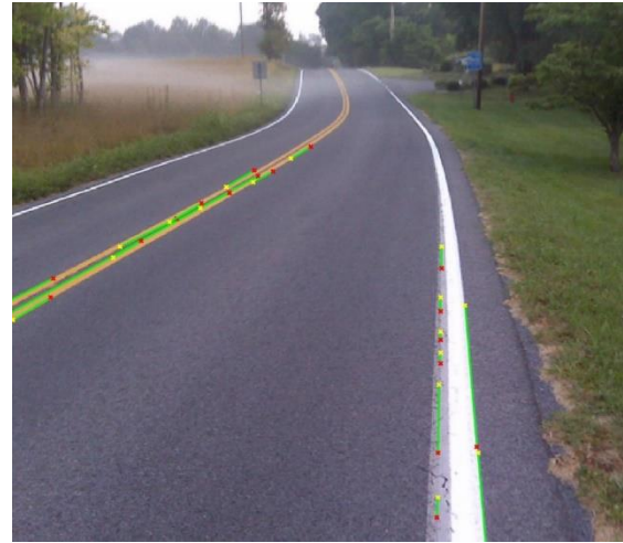
Figure 3: Edge Detection-Based Lane Detection Results
