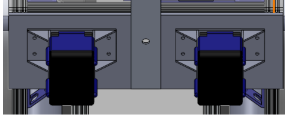
Figure 6. Dual Batteries allow Hot Swapping.
