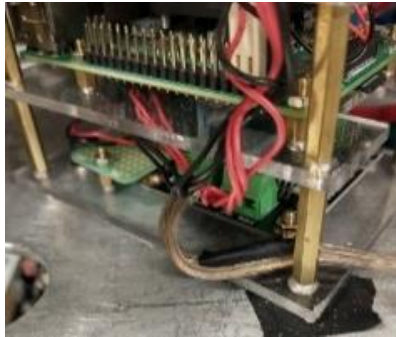
Figure 10a. Raspberry Pi Mount.
