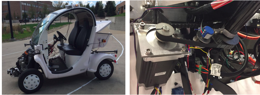
Drive-by-wire test runs with joystick game controller
