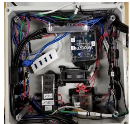
Figure 17: Internal Top View of Main Computer Case
