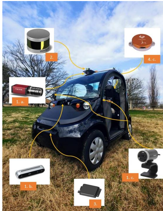
Figure 5. Sensor locations in the vehicle.
