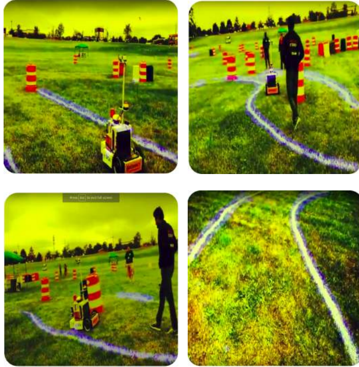
Figure 12: Lane Detections (Raw outputs from the network) illustrated in the blue channel. Test Image From: SeDriCa, Indian Institute of Technology Bombay, IGVC 2017 Winning Run
