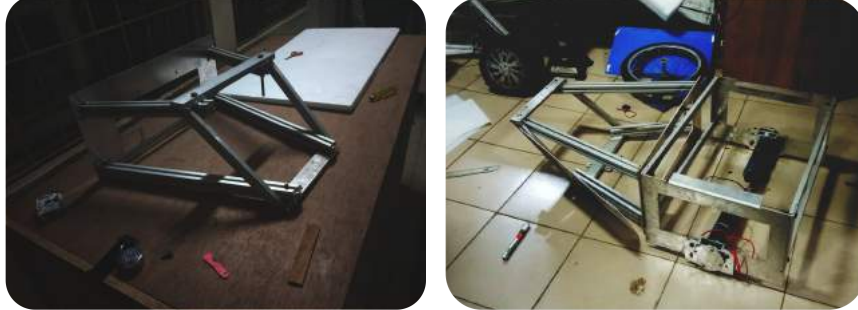
Figure 4: Front portion manufacturing and Total Chassis.
