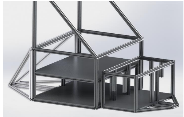
Figure 5: Capella Frame Structure
