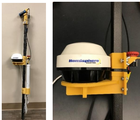
Figure 3: Sensor pole with close-up of 3D printed mounts
