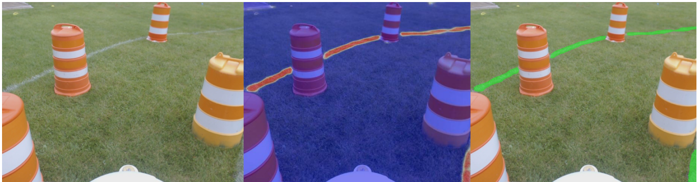
Figure 8: (Left) Original input image, (center) heat map of probability of a line from the CNN, and (right) the thresholded output of the CNN. This result is very promising given the lack of false negatives, particularly on the white stripes of the barrel (a previous weak point).
