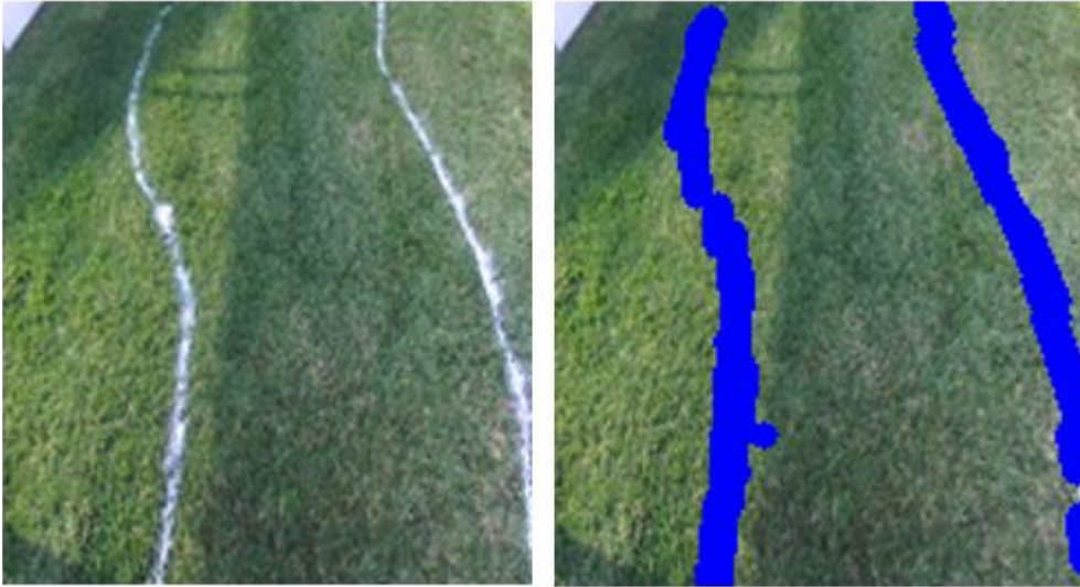
Figure 6: Example of Line Detection using Prepared Image
