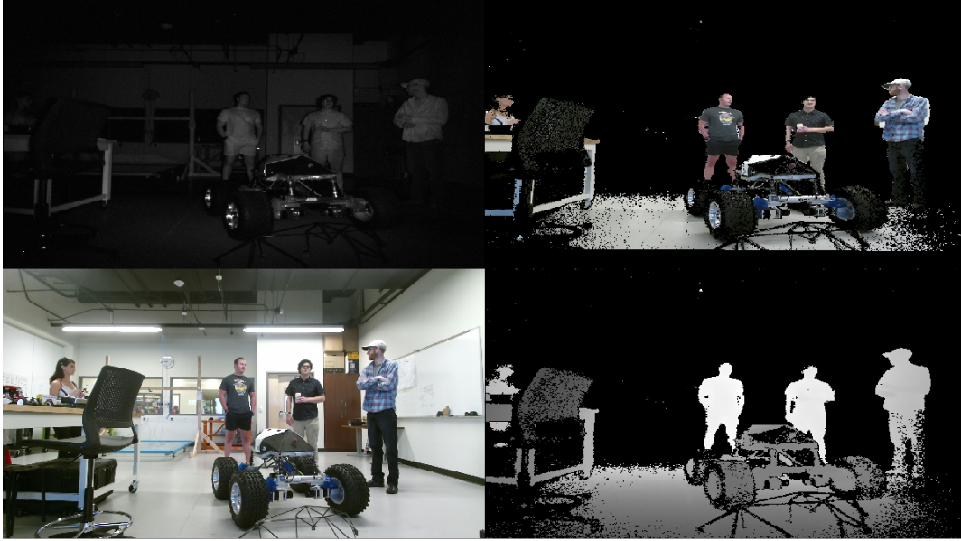
Figure 8: Live stream capture from Renegade rendering infrared, optical, and depth registration
