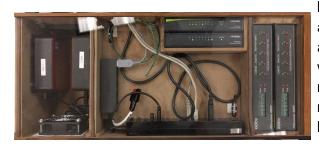
hubs are located within the box. Special attention was given to the thermal, cable, and power needs of each component within the box. The optimized layout reduced the total footage of cable on the robot as well as increased serviceability by making components easily removeable
