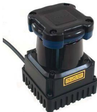
Figure 2: Measurement system : Hokuyo UTM-30LX-EW
