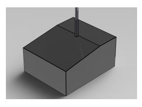
New to Dokalman this year is the addition of an acrylic shell, replacing the previous year's shell that was constructed from luan. This updated shell utilizes more standard shapes and designs. This design eased fabrication, eliminated areas for potential gaps, and therefore improved water resistance and allowed greater access the electronic components. The panels are mounted using thumb screws with brass thread-inserts set
