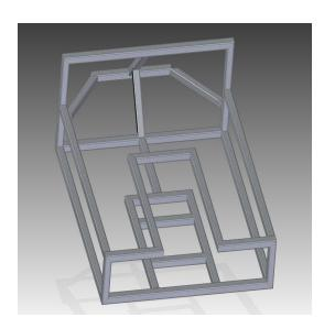
an optimal design for the rear of the robot that balanced strength and weight reduction. The frame was designed as a multi-level rectangular prism to house and protect the components in a balanced fashion. A triangular tail in the back fastened the caster wheels. This frame was welded together from 41-30 alloy steel tubing.
