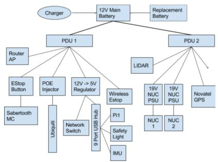
The electrical diagram to the left describes the hierarchy of powered devices in the robot. Each line off the PDU can be individually measured and disabled.
