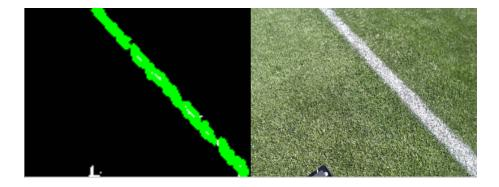
The main issue we faced at last years competition was that the vision algorithms that were employed could not properly handle dynamic lighting conditions. With lane detection being fundamental to the competition, this was a considerable complication. This has been a particular focus of ours for this year's competition.
