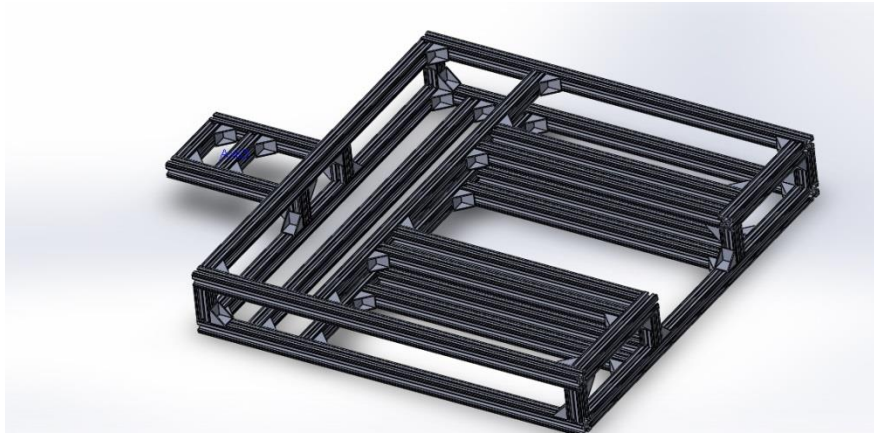
Fig.3 The complete frame designed using aluminium extrusion channels. Notice the right-angle joints are connected using angle brackets or by tapping the channels and using T-bolts.
