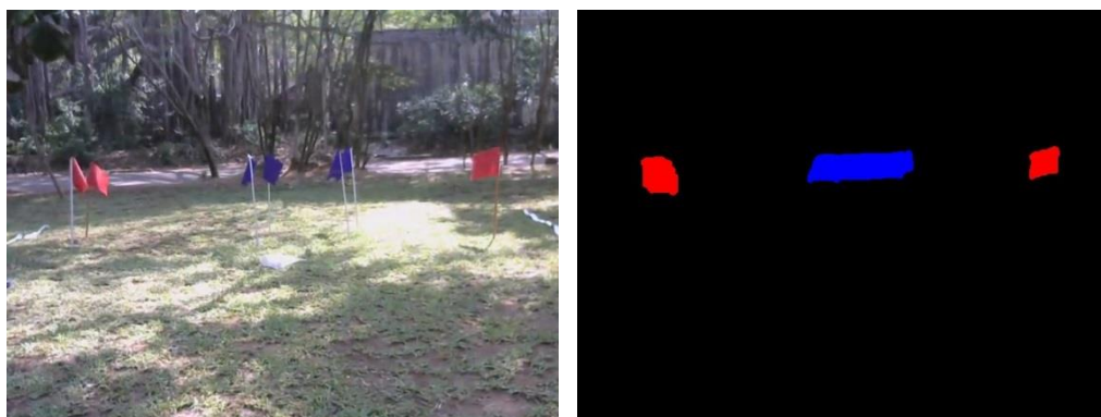
Fig. 19 Flag detection a) Original image b) Red and blue flags detected as continuous contours
