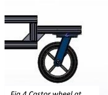
Fig.4 Castor wheel at rear of the vehicle
