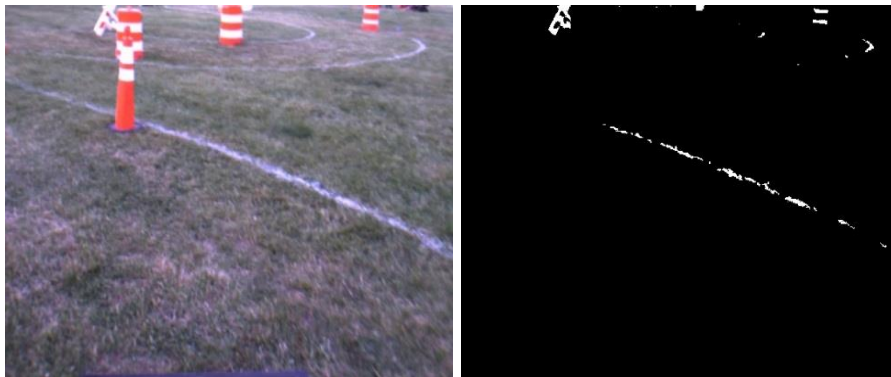
Fig. 17 Lane detection after masking obstacles a) Original image b) Final image after processing
