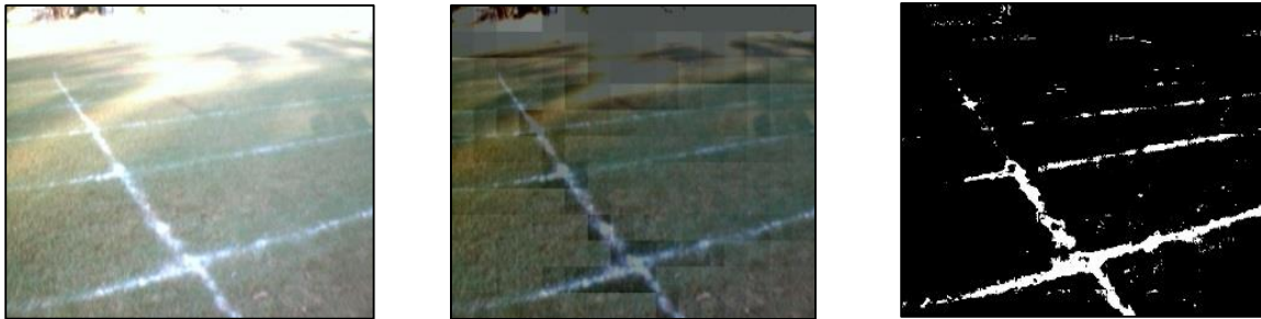
Figure 13. Illumination correction - Discrete Cosine Transform
