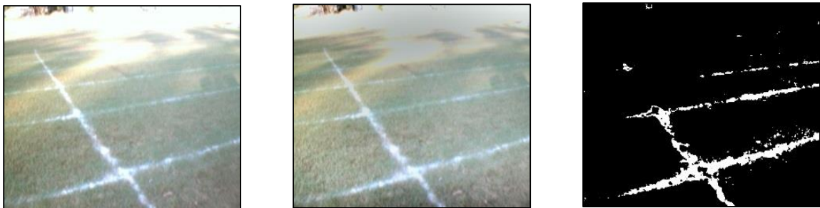
Figure 12. Illumination correction – Homomorphic Filtering
