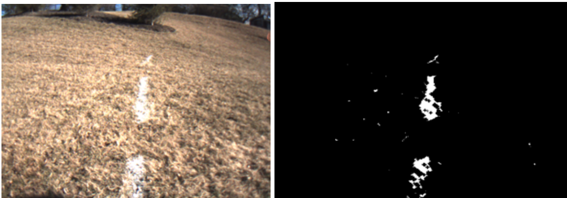
Figure 12 - White Line Detection - Original Image (Left) and Thresholded Image (Right)
