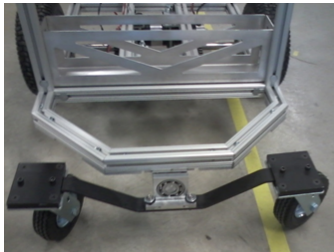
Figure 5 – The suspension system designed to stabilize the vision of the cameras
