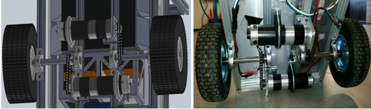
Figure 4 - The Solidworks model of the designed drivetrain
