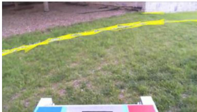
Figure 8.5: Lane Detection Result for Test Image. The above image demonstrates the results of the Hough transform conducted on the final edge image given by Figure 8.4. As expected, it detects the lane and accounts for changing geometries.
