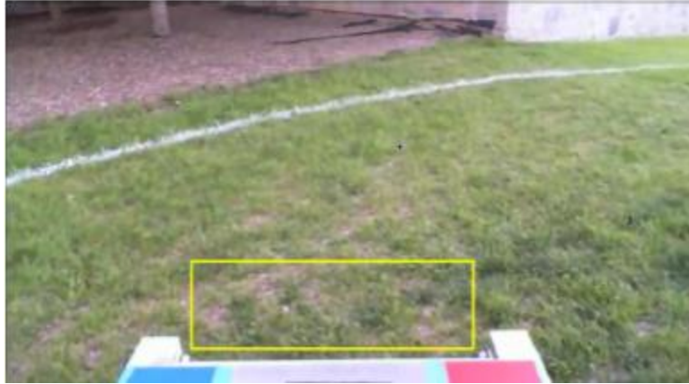
Figure 8.1: Grass Sample. The above figure demonstrates the area of sampling that is deemed grass. By assumption of the robot maintaining a certain distance from the line, this portion is sampled to determine the true grass properties in the current lighting.
