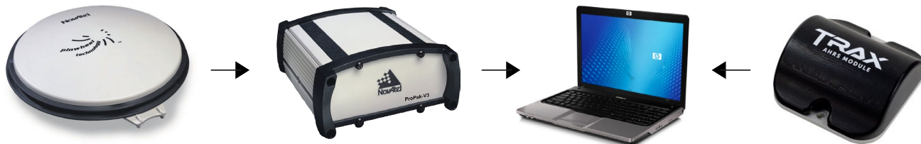
Figure 11: Navigation flowchart [from left to right: GPS antenna, GPS receiver, computer, compass]
