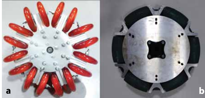
Figure 2: Comparison between previous platform wheels (a) with Yoshimi's new wheels (b).
