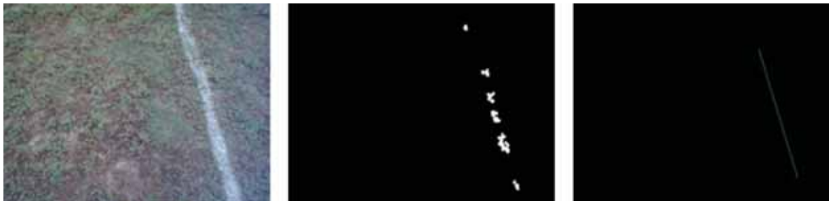
Figure 10: Lane detection using color thresholding.
