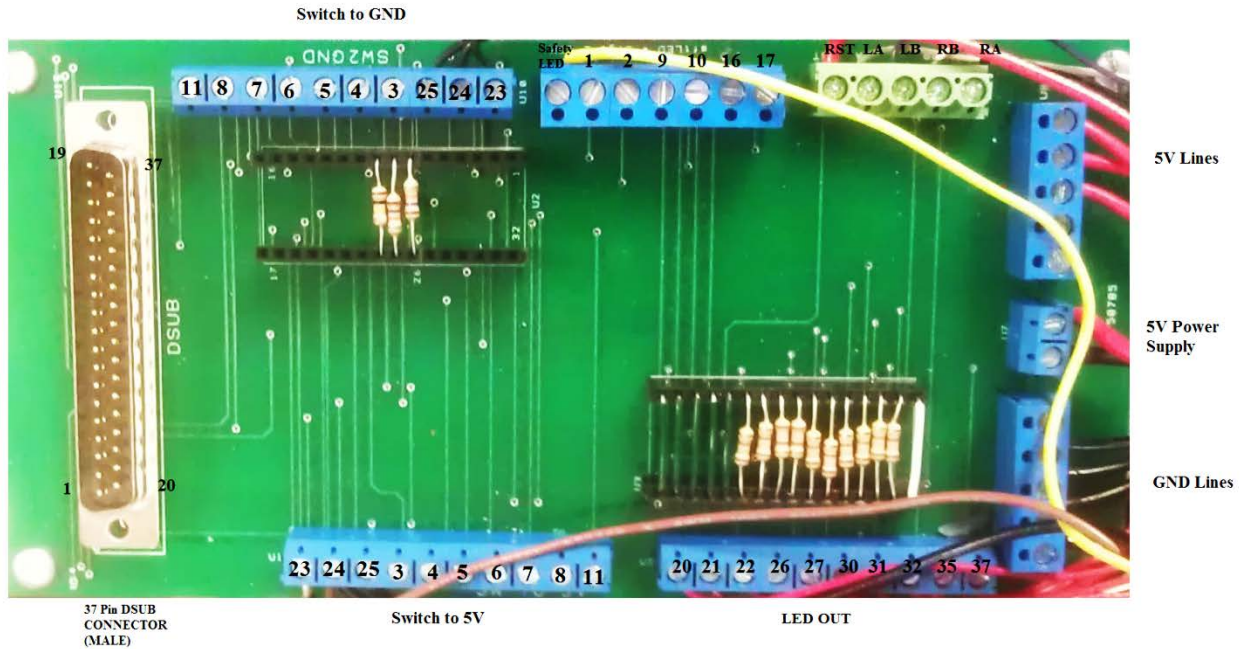
Figure 6: Printed Circuit Board (PCB) for the Front Panel Controller.
