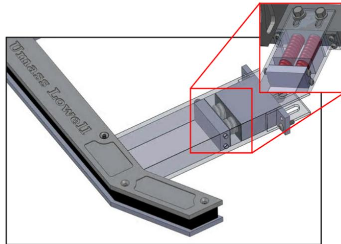
Figure 4: Spring Dampened Bumper
