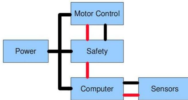
Figure 9: Electrical System Layout (Black = Power, Red = Data)
