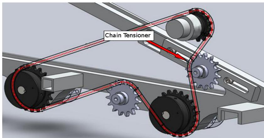
*Figure 3: One Side of Stark's Drive-train*
