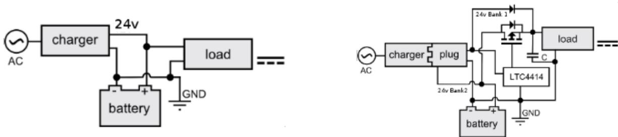
Figures 10: Old Charging Circuit and New Charging Circuit (left to right)
