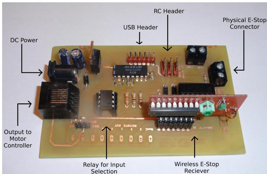
*Figure 12: Motor Controller Interface*
