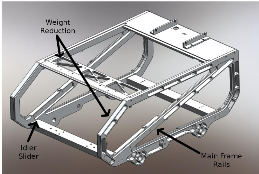
*Figure 2: Key Points of Stark's Frame*
