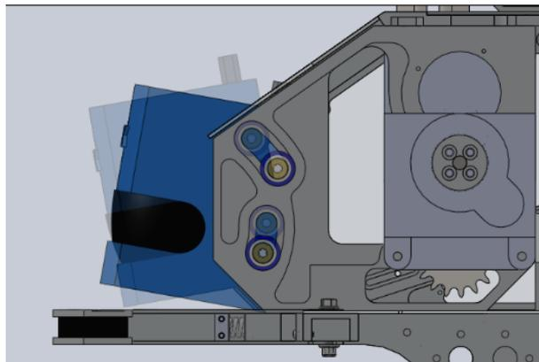
*Figure 8: SICK Laser Mount*
