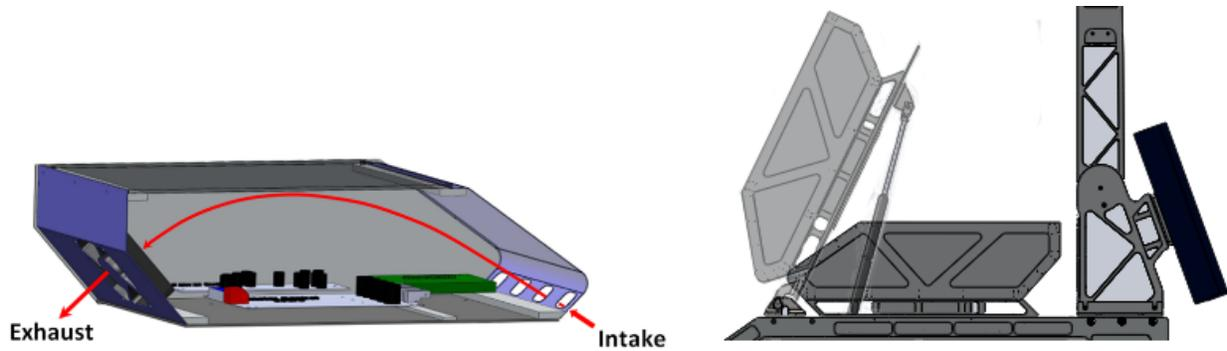
*Figure 7: Control Box Air Flow, Control Box Positions*
