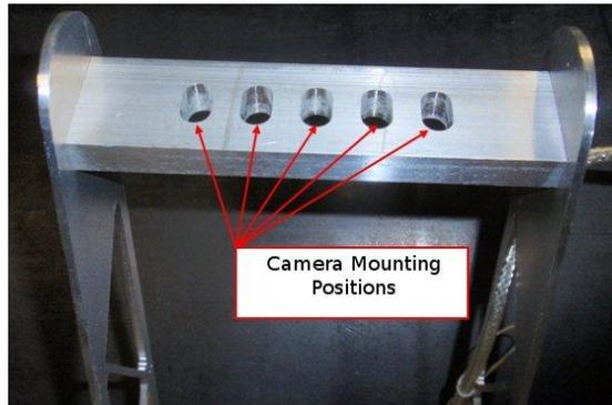
*Figure 5: Camera Mounts on Sensor Mast*
