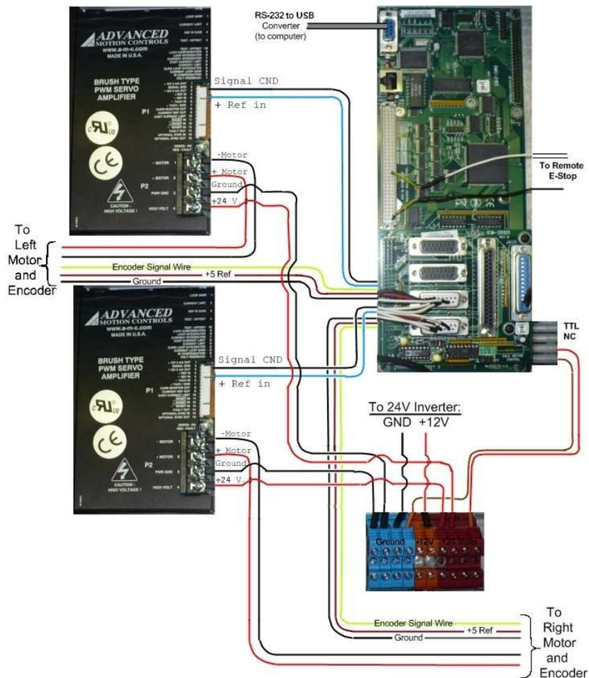
Figure 5: Wiring Diagram for CAT Motion Controls
