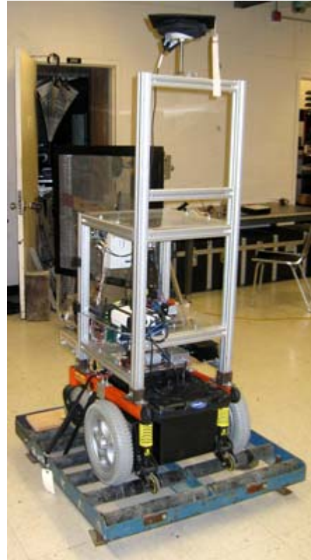
Figure 1 - Partially constructed Harlie used for testing mechanical structure and wiring against vibration damage.
