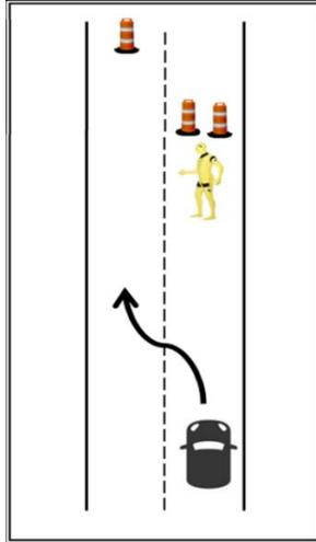
**Figure 18: Functions Testing. Pedestrian Detection. Lane Changing**
