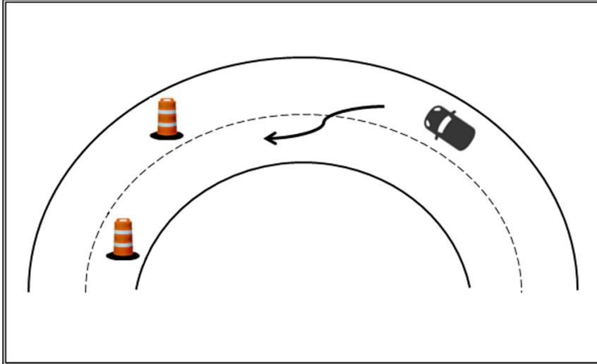
**Figure 21: Functions Testing. Curved Road Evaluation. Lane Changing**
