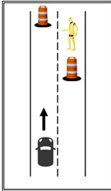
**Figure 17: Functions Testing. Obstructed Dynamic Pedestrian Detection**
